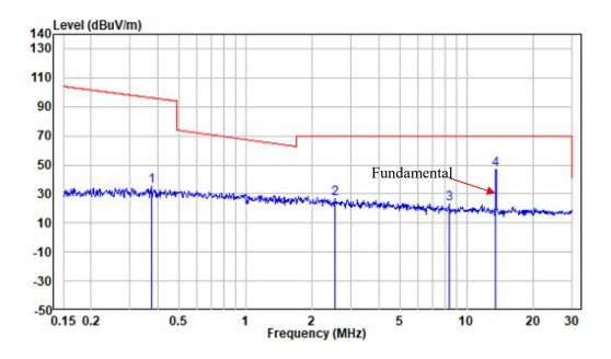
Site : chamber Condition: 3m Job No. : RA221201-58353E-RF Test Mode: NFC Note : Ground-parallel
