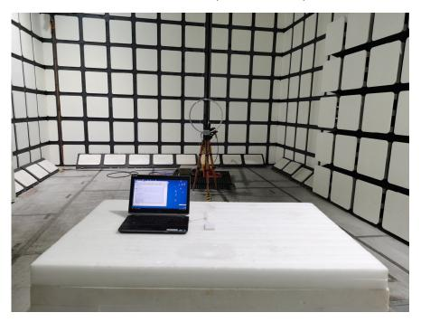
Radiated Emissions View (9 kHz-30 MHz) -Ground-parallel
