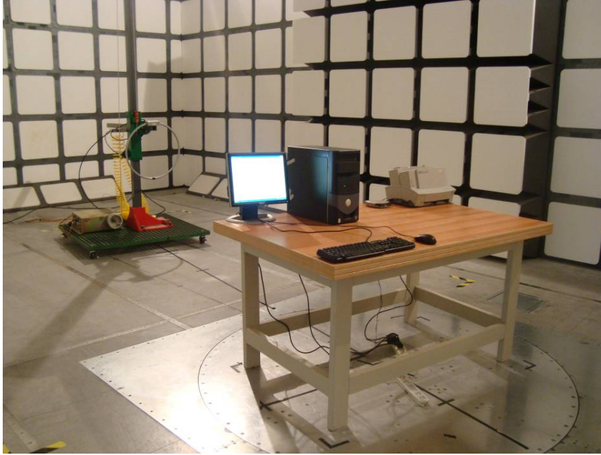
Below 30MHz: Radiated Emissions - Front View
