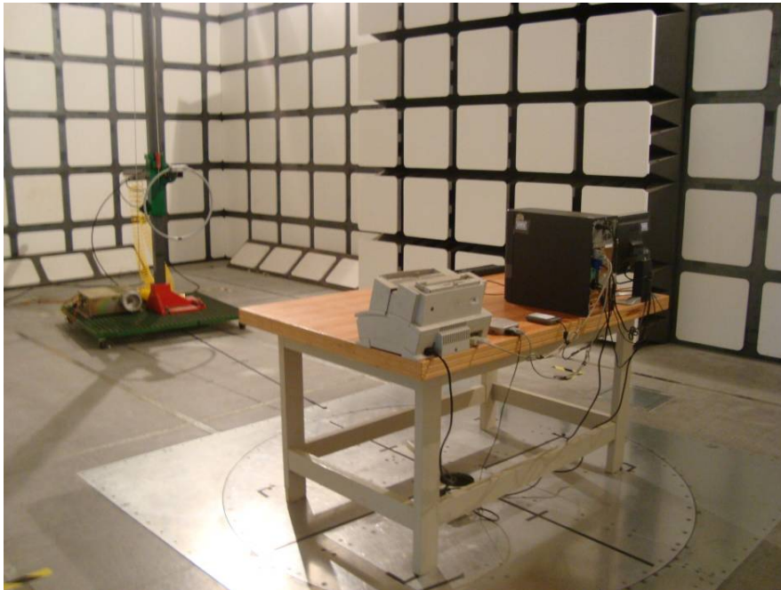
Below 30MHz: Radiated Emissions - Rear View
