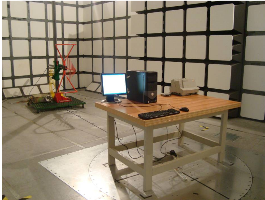
Above 30 MHz: Radiated Emissions - Front View
