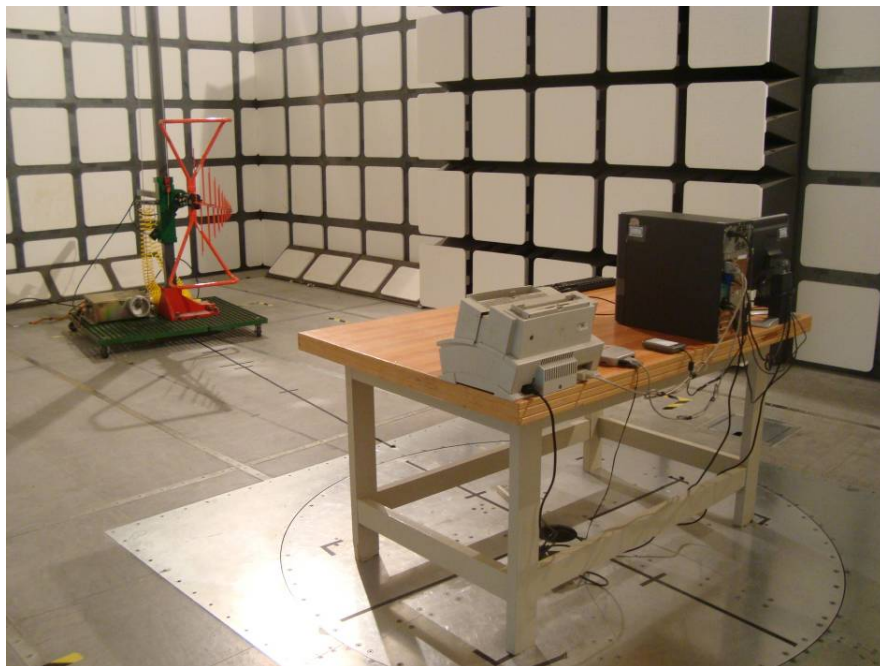
Above 30 MHz: Radiated Emissions - Rear View
