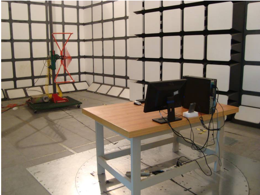
Above 30 MHz: Radiated Emissions - Rear View
