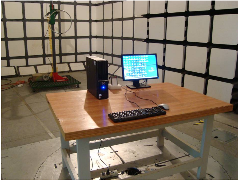
Below 30MHz: Radiated Emissions - Front View
