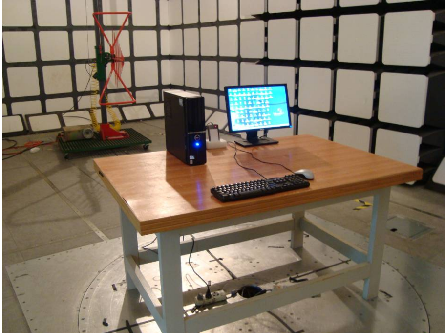
Above 30 MHz: Radiated Emissions - Front View
