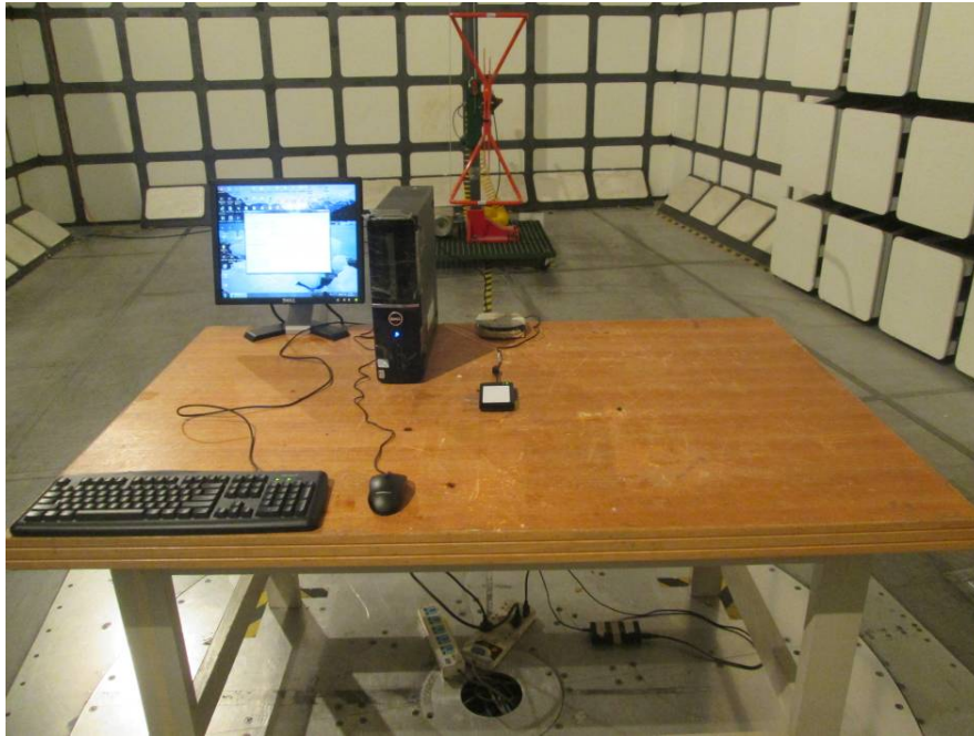
Radiated Emissions – Front View (Above 30 MHz)
