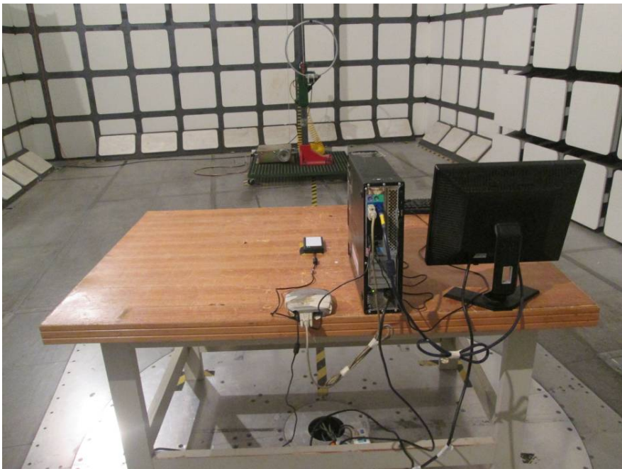
Radiated Emissions – Rear View (Below 30 MHz)
