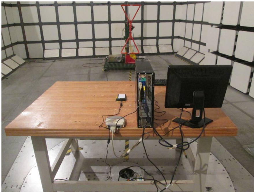
Radiated Emissions – Rear View (Above 30 MHz)
