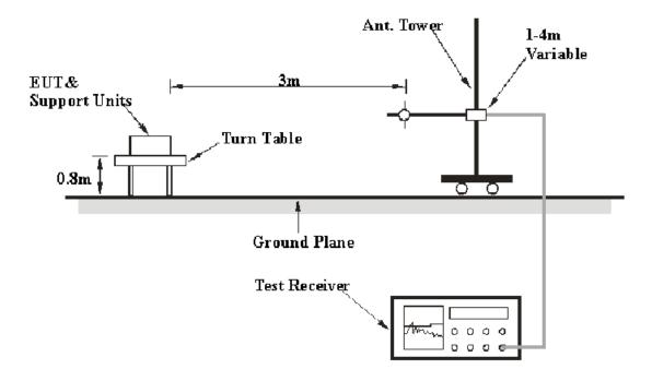
The radiated emission tests were performed in the 3-meter chamber A test site, using the setup accordance with the ANSI C63.4-2003. The specification used was the FCC Part Subpart C limits.
