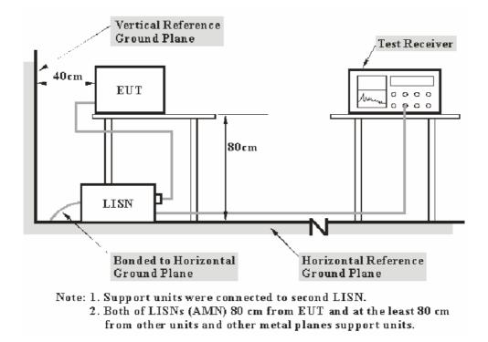
The setup of EUT is according with per ANSI C63.4-2003 measurement procedure. The specification used was with the FCC Part 15.207.
