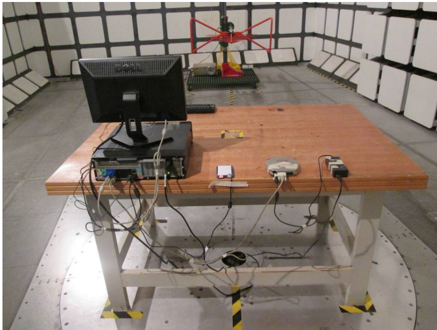
Radiated Emissions – Rear View (Above 30 MHz)
