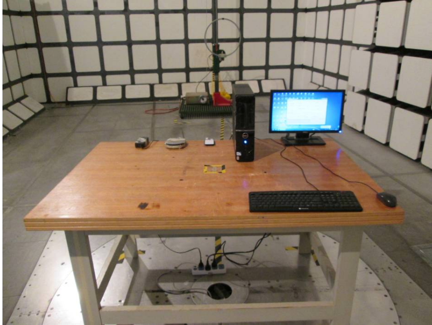
Radiated Emissions – Front View (Below 30 MHz)
