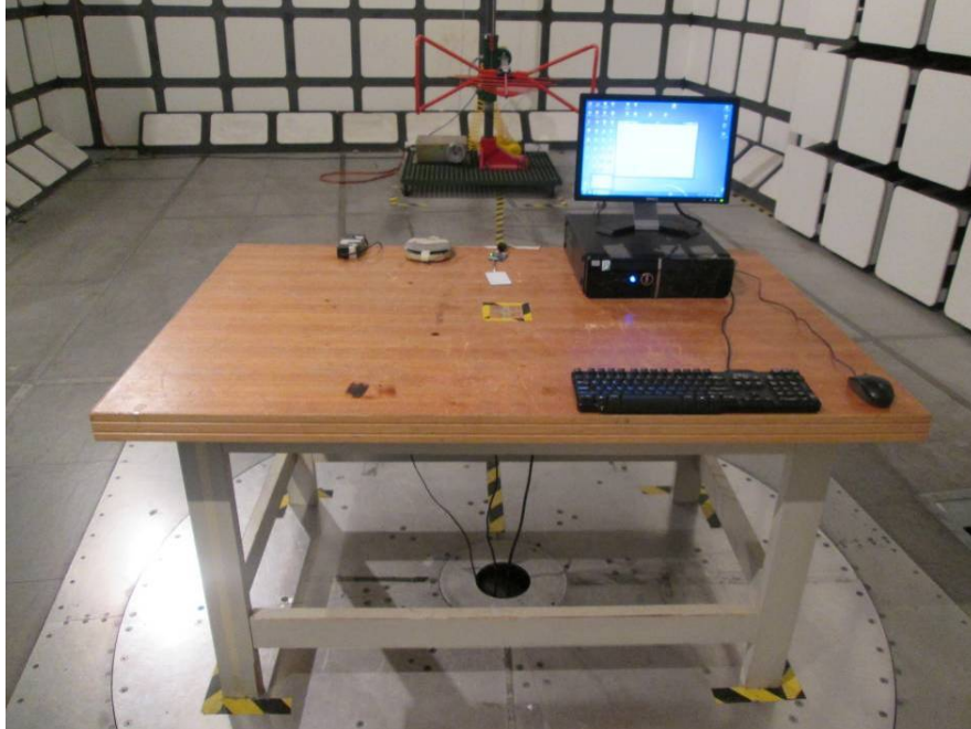
Radiated Emissions – Front View (Above 30 MHz)
