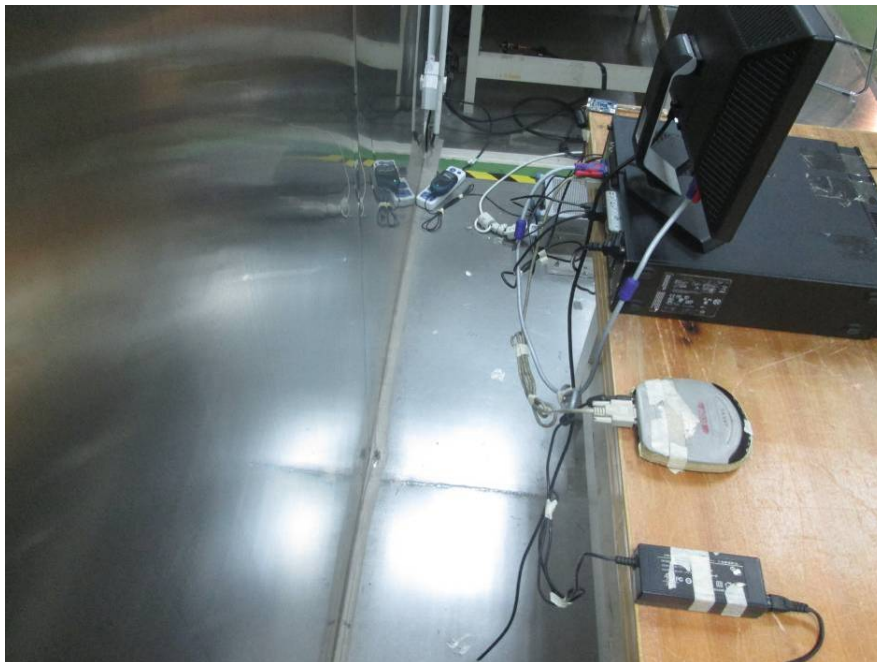
Conducted Emissions - Side View
