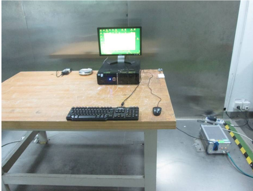
Conducted Emissions - Front View
