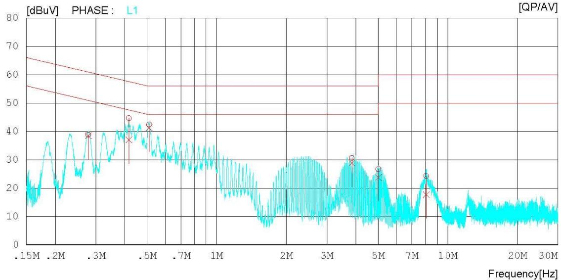
AC Line Conducted Emissions (List)&Modulation: GFSKResults of Conducted Emission
