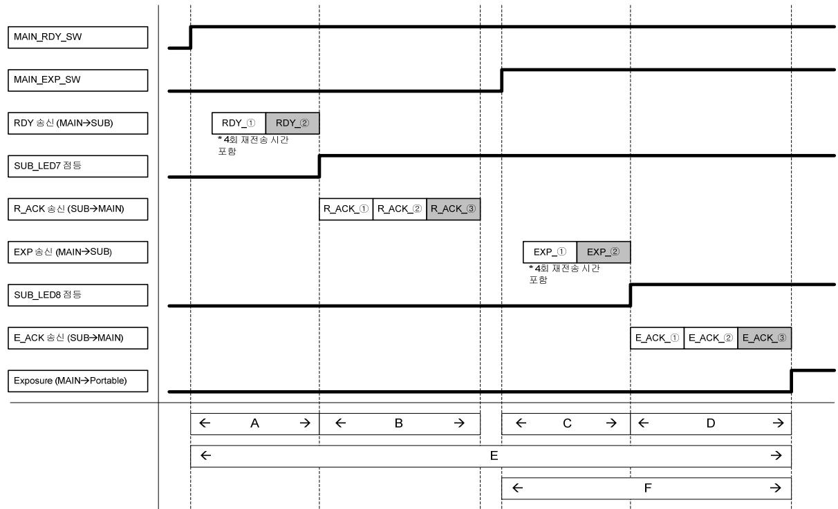
\*A section (Time : about 1060 ms) – Time from pushing Hand S/W Ready to RF SUB Ready LED action.
