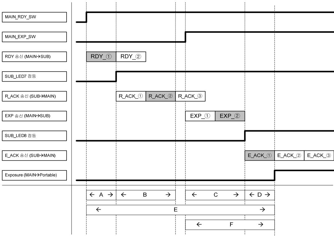
**\*A section** (Time : about 50 ms) – *Time from pushing Hand S/W Ready to RF SUB Ready LED action*
