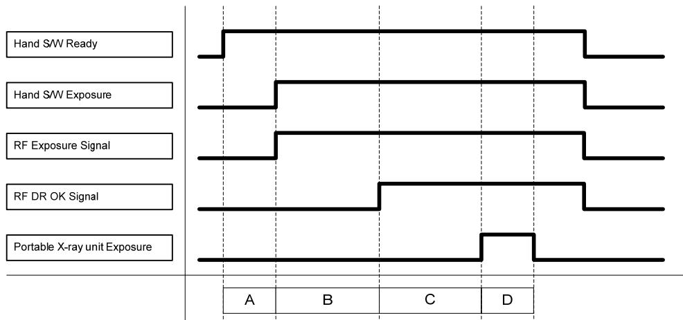
\***A section** (Time : about 1300 ms) – *Time from pushing Hand S/W Ready to finalizing Portable X-Ray Unit preheat.*
