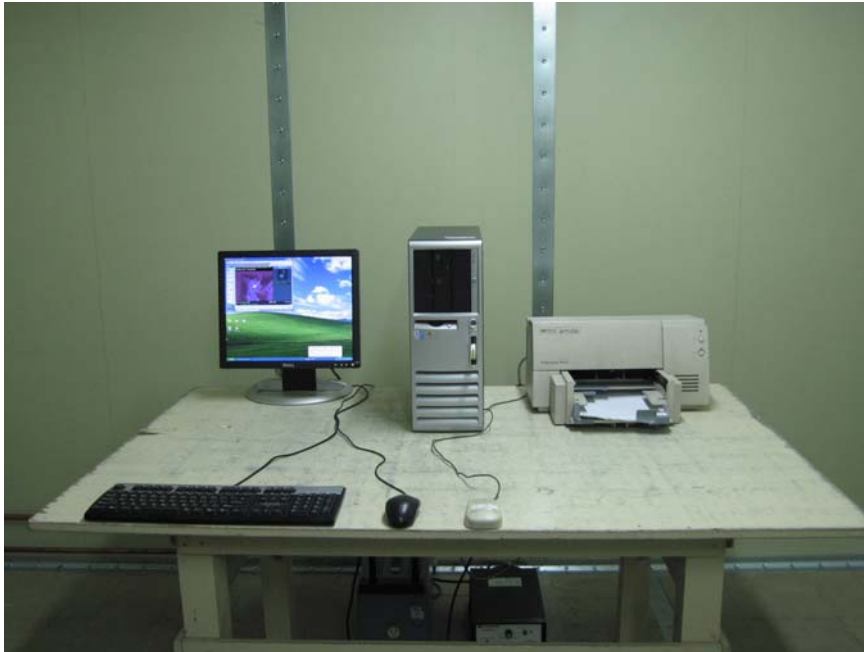
Photograph 2 : Setup for Conducted Emissions
