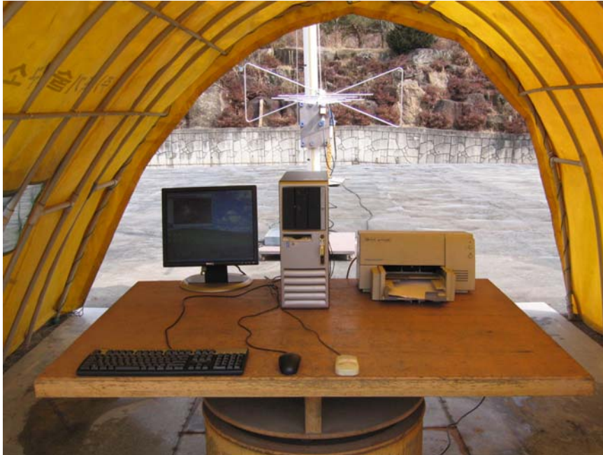
Photograph 1 : Setup for radiated Emissions
