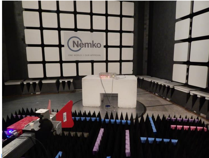
Figure 9.1-1: Radiated setup photo
