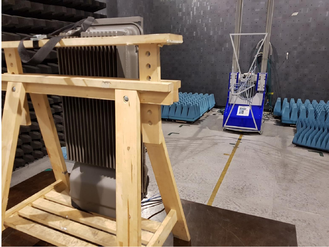
Test set up radiated emission 30 MHz – 1GHz
