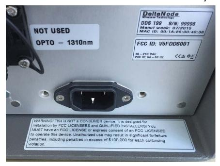
WARNING. This is NOT a CONSUMER device. It is designed for installation by FCC LICENSEES and QUALIFIED INSTALLERS. You MUST have an FCC LICENSE or express consent of an FCC Licensee to operate this device. Unauthorized use may result in significant forfeiture penalties, including penalties in excess of \$100,000 for each continuing violation.
