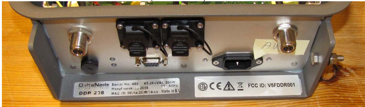
Bottom side with connectors and labels (AWS unit)
