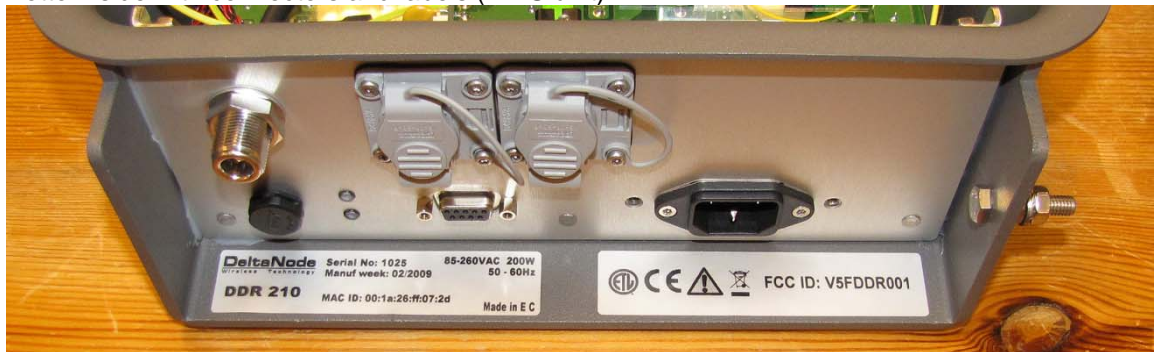
Bottom side with connectors and labels (AWS unit)
