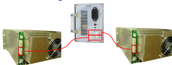
Backup Power for Two Master Units
