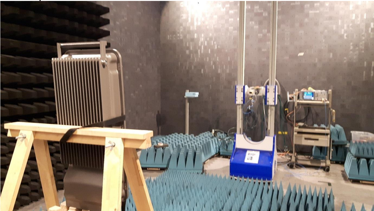
Test set up radiated emission 18 GHz – 27 GHz
