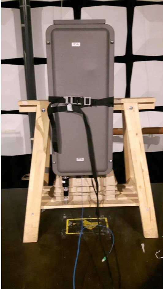
Test set up radiated emission 30 MHz – 1GHz
