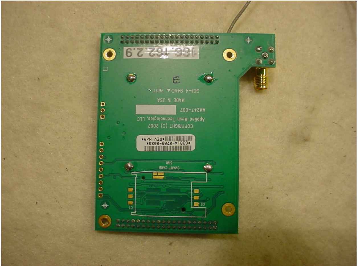
Figure 10: Internal Photos – DCX CDMA – Carrier Board Back
