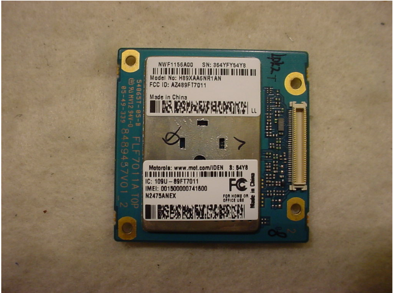
Figure 7: Internal Photos – DCX iDEN Internal/External Antenna – iDEN Module
