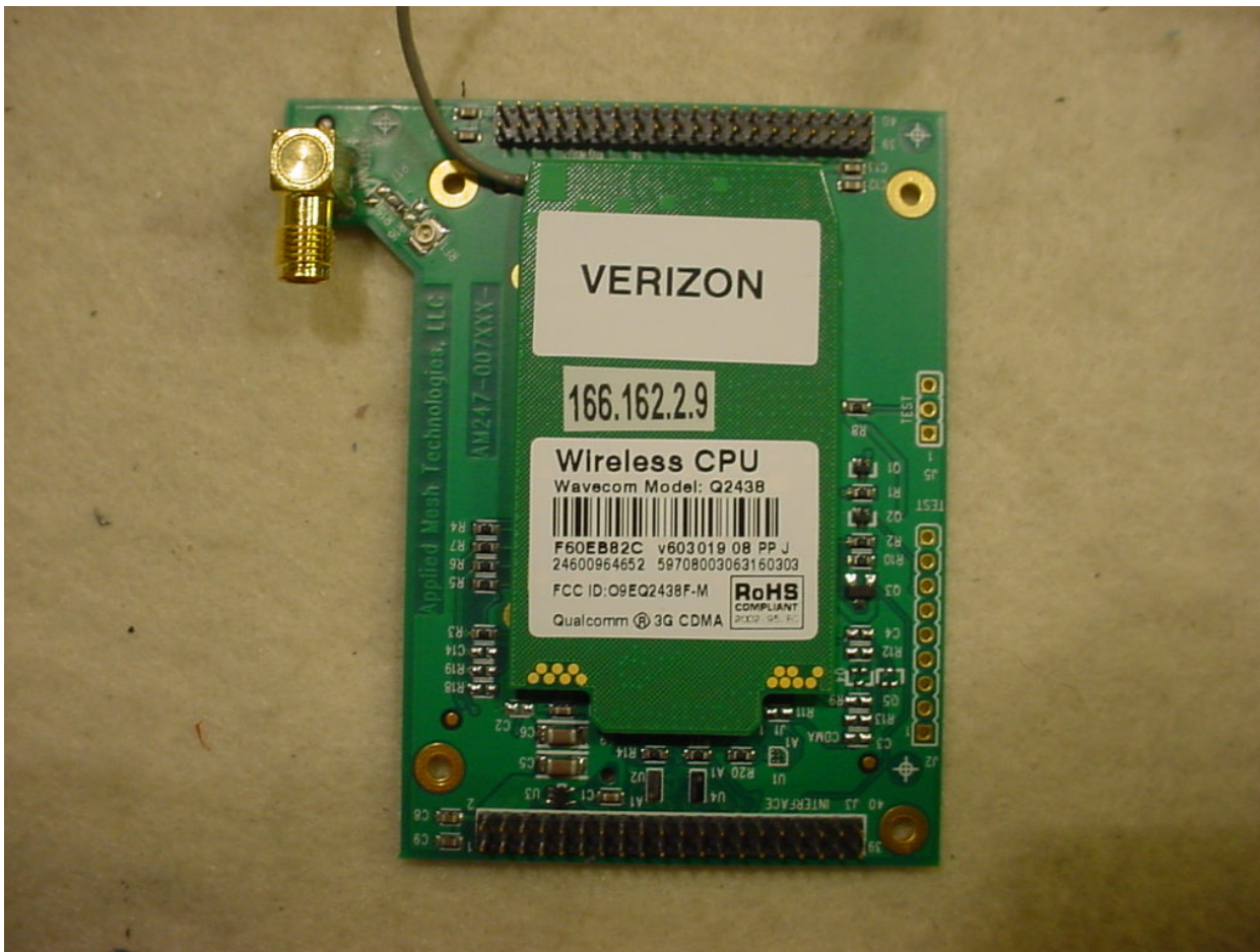
Figure 9: Internal Photos – DCX CDMA – Carrier Board Front
