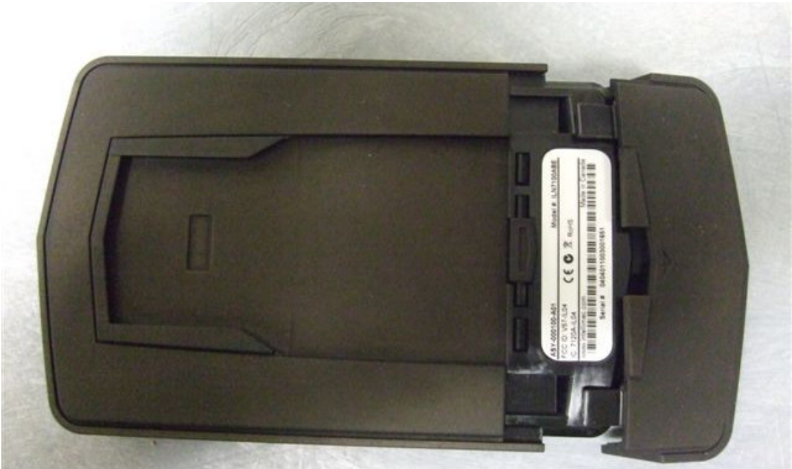
Fig. 4 iLane bottom cover completely removed, label exposed.
