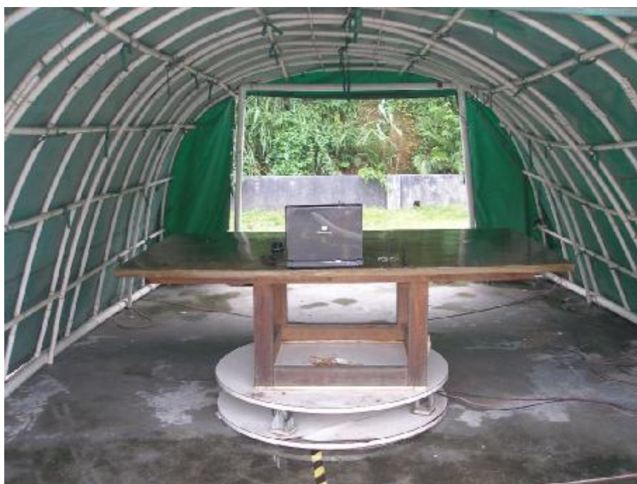
Radiated emission test view
