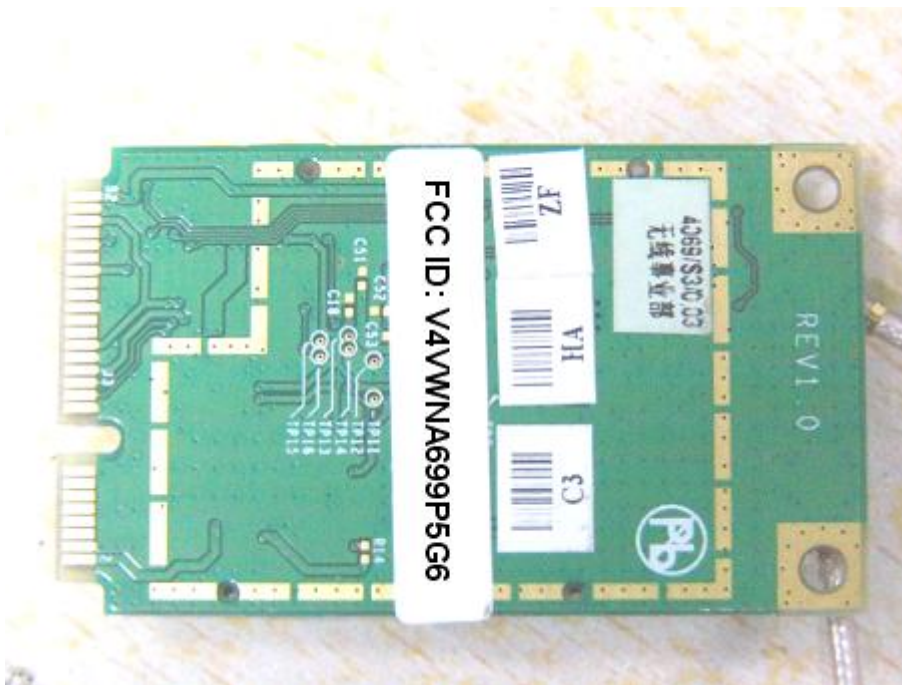
Main & RF board solder side
