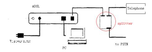
Splitter is a filter for the telephone. It can split the analog signal and the digital signal. The analog signal was send to the telephone, the digital signal was send to the ADSL. The splitter is make by capacity and inductance.
