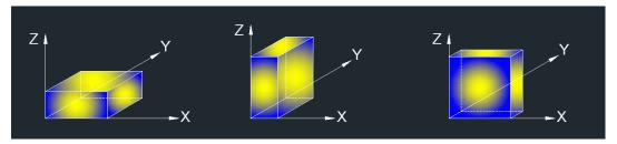
Note 1: The manufacturer has recommended that the EUT only be used in the desktop (horizontal) orientation; therefore, all radiated testing was performed in desktop orientation. The EUT was placed on normal orientation and all radiated emissions were performed with the EUT shown on the setup photo.
