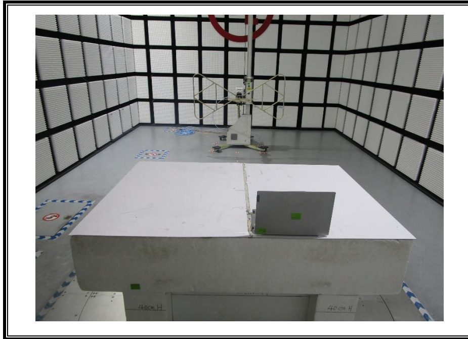
RADIATED RF MEASUREMENT SETUP (Below 30MHz)
