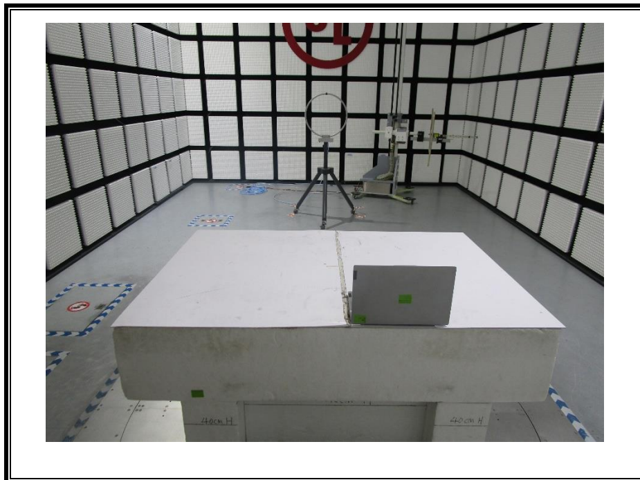
RADIATED RF MEASUREMENT SETUP (Below 30MHz)
