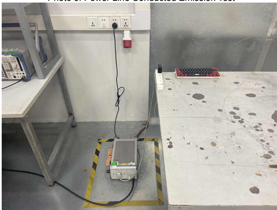
FCC ID: V4P-GM610 Photo of Power Line Conducted Emission Test
