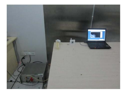
**Radiation Emission Test Setup (Below 30MHz)**
