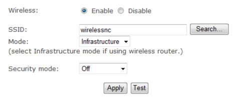
[SSID] Type the ID of the wireless network you want to connect to using up to 32 ASC  ${\tt II}$  characters or click **Search** to search for available networks.
