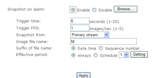
[Trigger time] How many seconds does camera keep snapshot the images after get a motion alarm.
