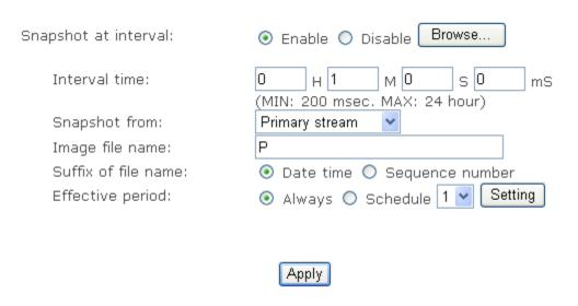
**[Interval time]** Type the interval at which you want to save snapshot to SD card periodically. **[Snapshot from]** Select stream that snapshot from.
