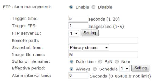
[Trigger time] How many seconds does camera keep snapshot the images after get a motion alarm.
