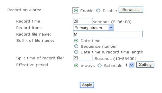
[Recordr time] how many seconds does camera keep recording after a motion alarm.
