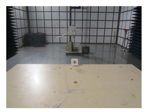
Radiation Emission Test Setup (Above 1GHz)
