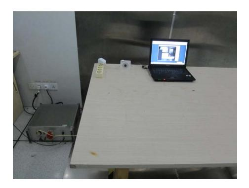
Radiation Emission Test Setup (Below 30MHz)
