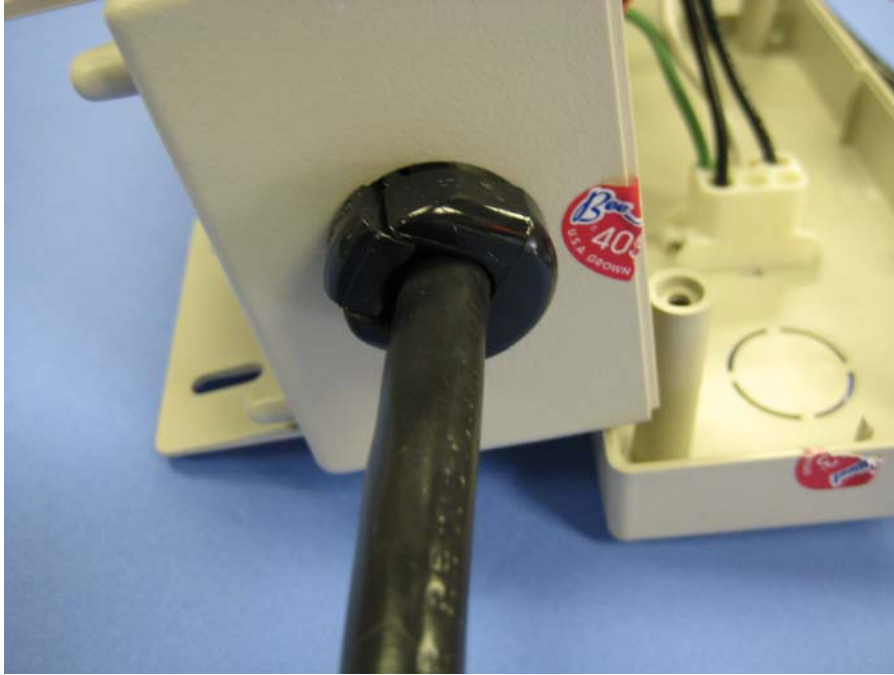
View of External Connection Point for Cable
