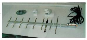
The components shown in the picture above are a one (1) inch pipe flange, a 2 ½ foot piece of 1" PVC schedule 40 pipe, a male socket adapter, and if required a one in 90 degree male thread and socket combination. These items are available at any local hardware store.
