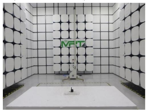
Description: Radiated disturbance Test Setup for Above 1GHz
