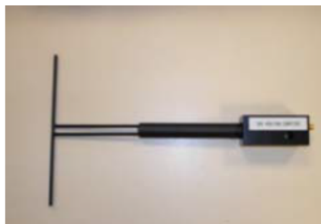
Figure 1 – Satimo COMOSAR Validation Dipole
