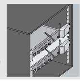
Fitting the receiver in a 19" rack. Leave one unit space free between two receivers in the rack.
