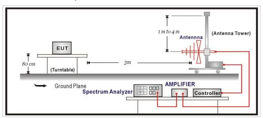
Above 1GHz Test Setup:
