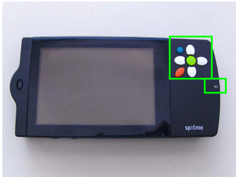
Front of Unit, "screen closed" Screen, Top Keypad Keys (7 buttons), LED
