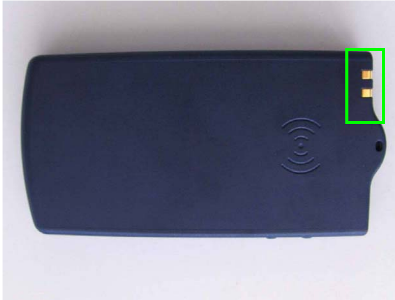
Rear of Unit, "screen closed" Charge Contacts (2 contacts)
