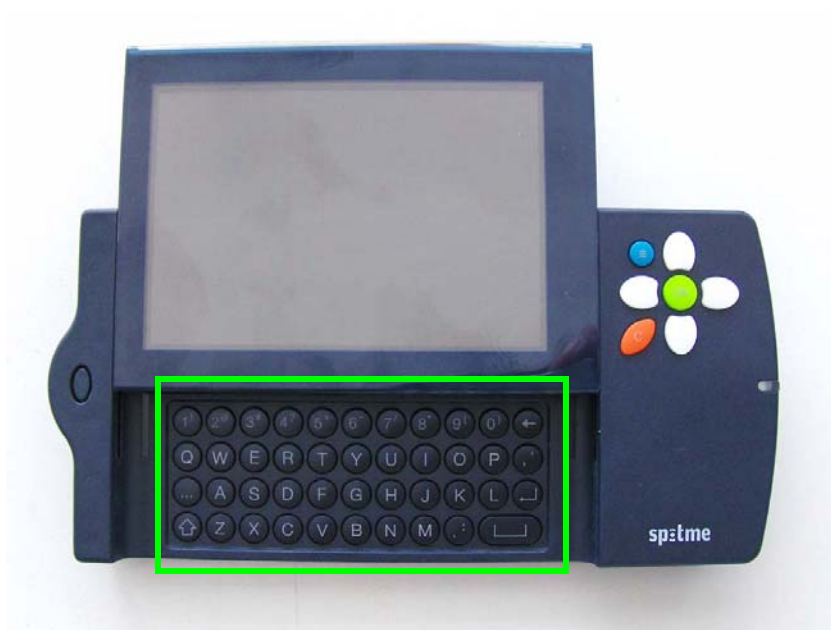
Front of Unit, "screen opened" Bottom Keypad Keys (QWERTY)
