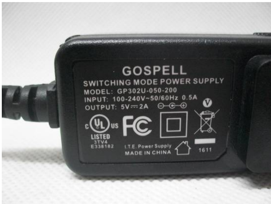
PHOTO OF POWER SUPPLY2
