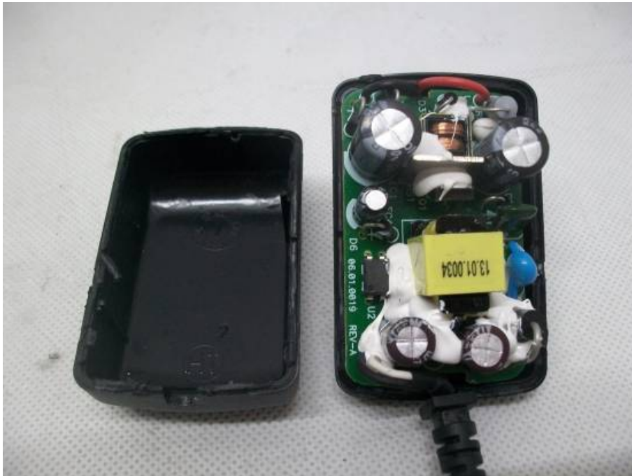
INTERNAL PHOTO OF POWER SUPPLY1 - 1
