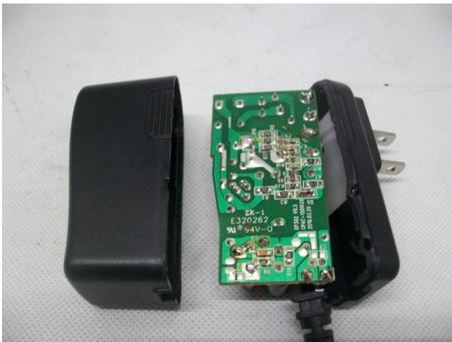
INTERNAL PHOTO OF POWER SUPPLY2 - 1
