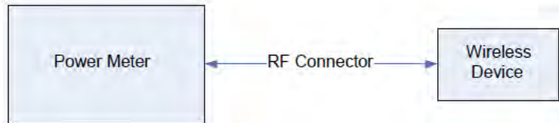
Figure 6.3.1 Power Measurement Setup
