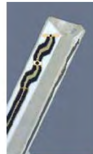
Figure E.2.2 Probe Thick-Film Technique
