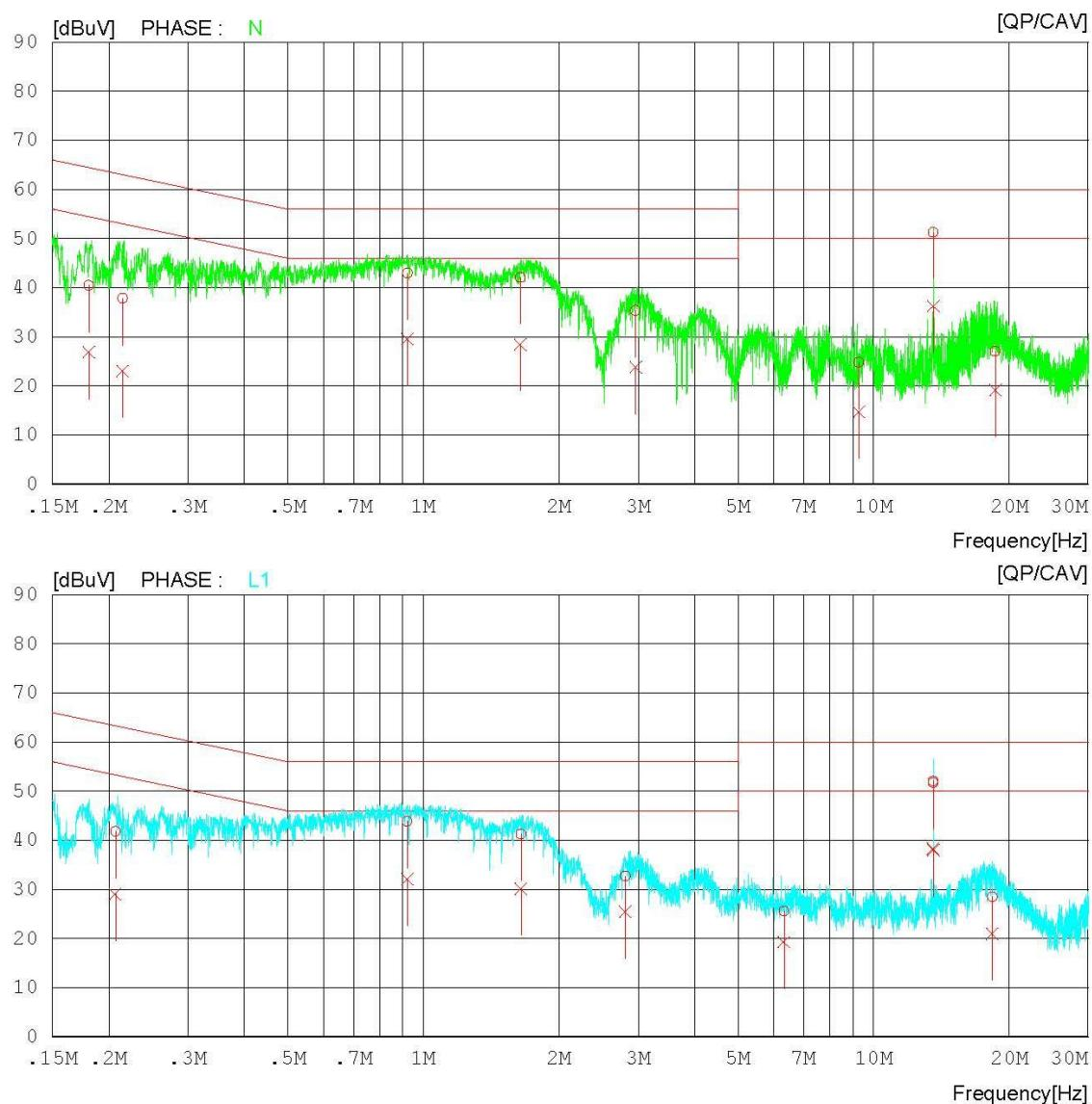
**Measurement Data****Results of Conducted Emission**
