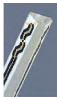
Figure E.2.2 Probe Thick-Film Technique
