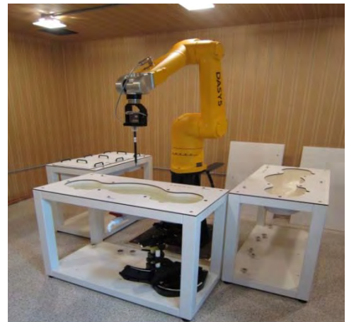
Figure E.7.1 DASY5 Test System
