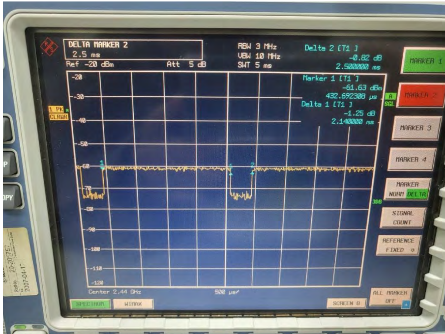
Figure 8.2.4 Bluetooth Transmission Plot
