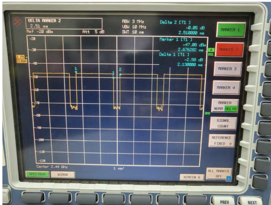
Figure 8.2.3 Bluetooth Transmission Plot
