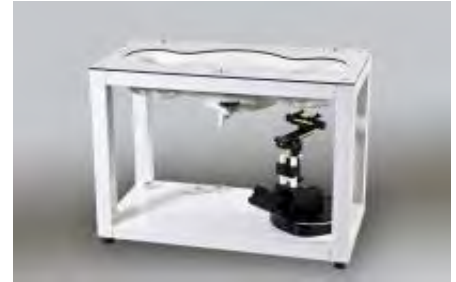
Figure E.5.1 SAM Twin Phantom
