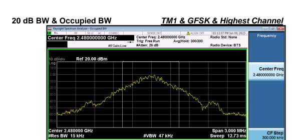
**Total Power** 10.0 dBm Occupied Bandwidth 885.70 kHz Frea Offset **Transmit Freq Error** -10.201 kHz % of OBW Power 99.00 % x dB Bandwidth 887.9 kHz x dB -20.00 dB
