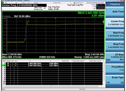
Number of Hopping Channels 2(FH) <u>Hopping mode : Enable & TM1 &π/4DQPSK</u>
