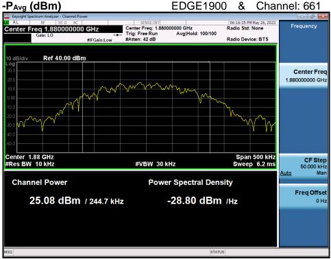
PAPR (dB) =  $P_{Pk}$  (dBm) -  $P_{Avg}$  (dBm) = 29.06 dBm - 25.08 dBm = 3.98 dB
