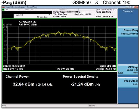
PAPR (dB) =  $P_{Pk}$  (dBm) -  $P_{Avg}$  (dBm) = 32.77 dBm - 32.64 dBm = 0.13 dB
