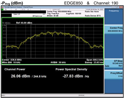
PAPR (dB) =  $P_{Pk}$  (dBm) -  $P_{Avg}$  (dBm) = 29.27 dBm - 26.06 dBm = 3.21 dB
