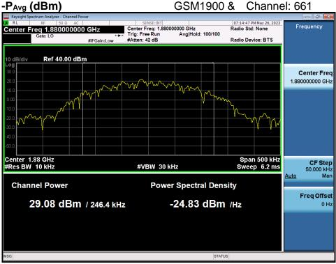
PAPR (dB) =  $P_{Pk}$  (dBm) -  $P_{Avg}$  (dBm) = 29.27 dBm - 29.08 dBm = 0.19 dB
