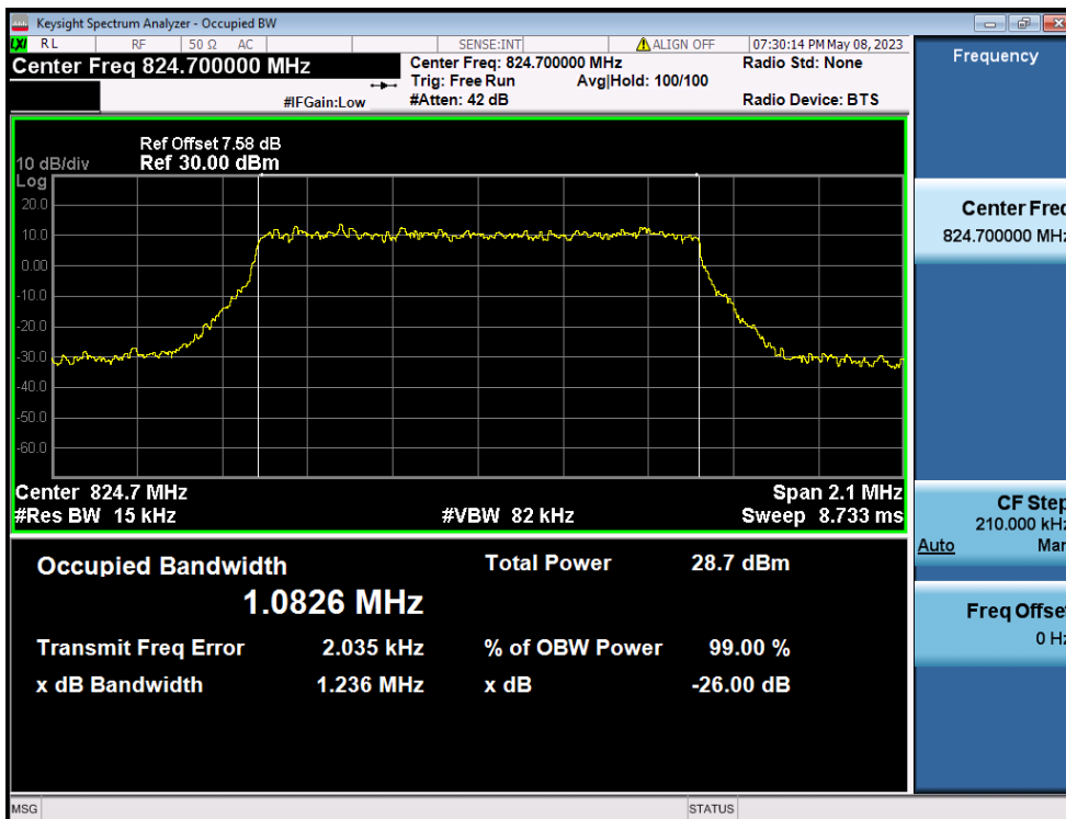
LTE Band 26(5) / 1.4MHz / 16QAM - RB Size 6
