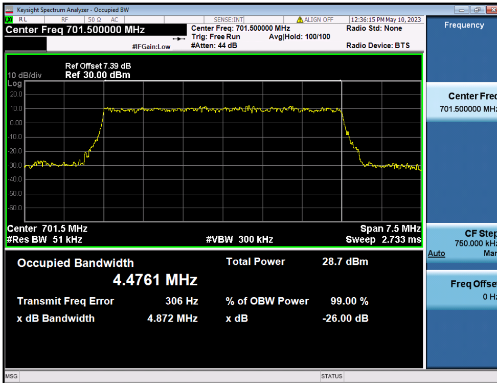
LTE Band 12(17) / 5MHz / 16QAM - RB Size 25
