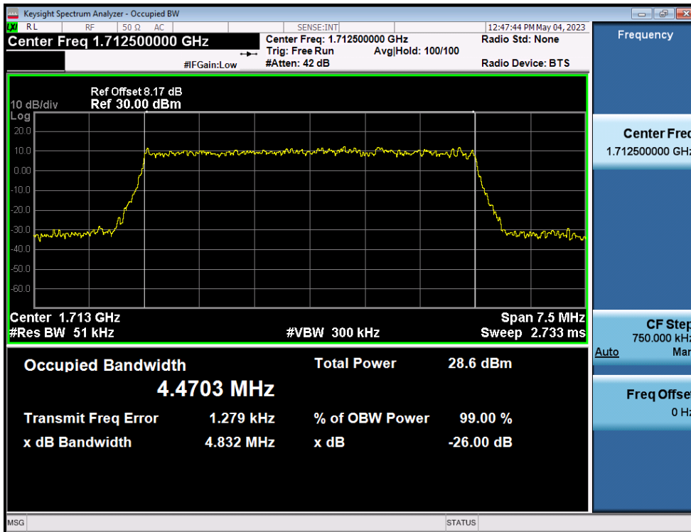
LTE Band 66(4) / 5MHz / 16QAM - RB Size 25
