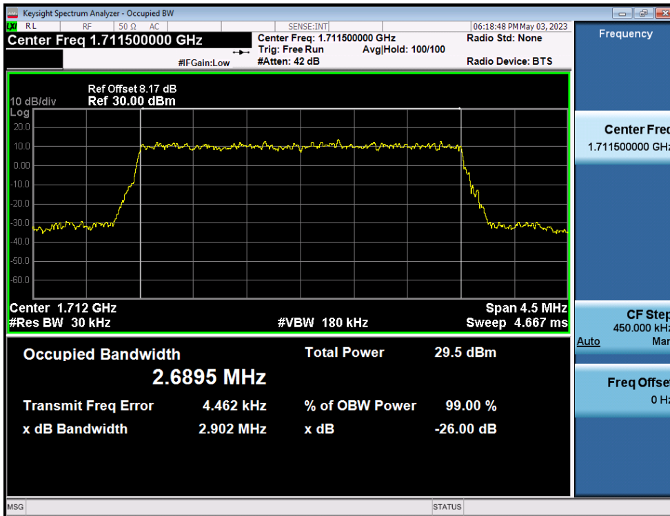
LTE Band 66(4) / 3MHz / QPSK - RB Size 15
