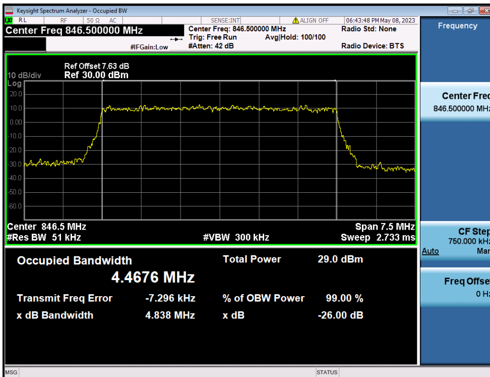
LTE Band 26(5) / 5MHz / 16QAM - RB Size 25
