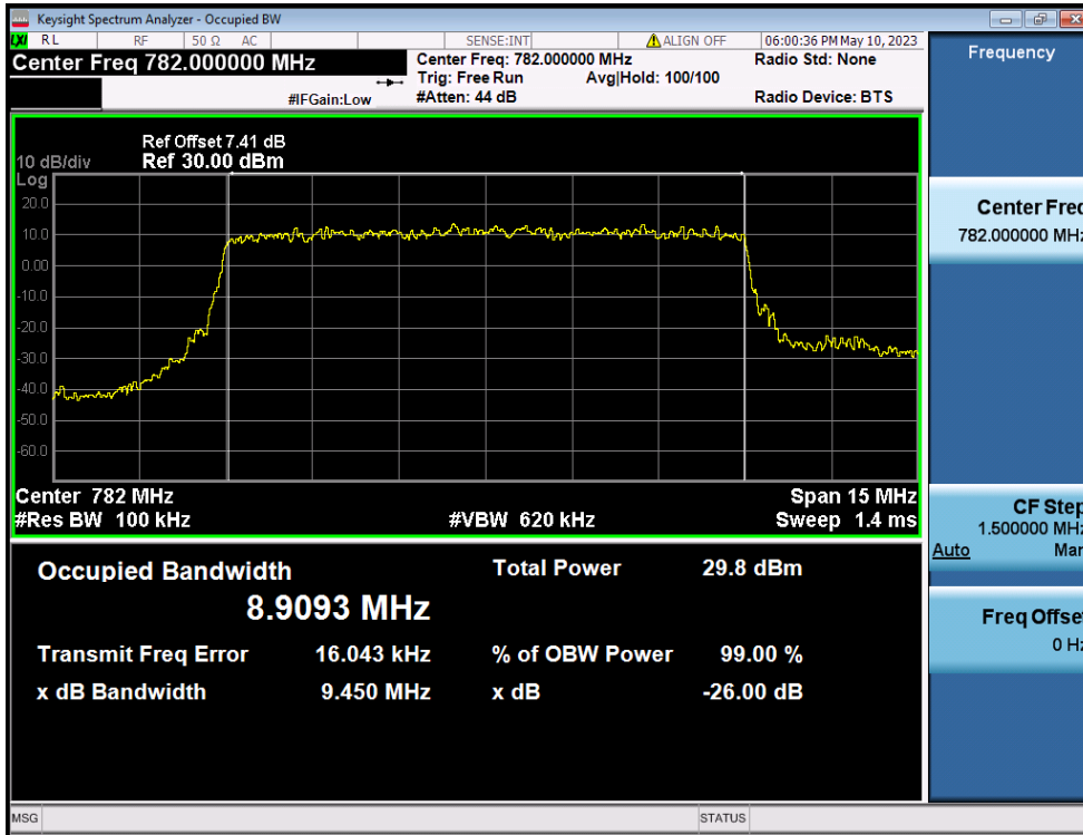
LTE Band 13 / 10MHz / QPSK - RB Size 50
