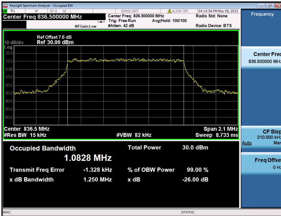
LTE Band 26(5) / 1.4MHz / QPSK - RB Size 6
