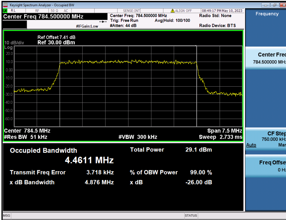
LTE Band 13 / 5MHz / 16QAM - RB Size 25
