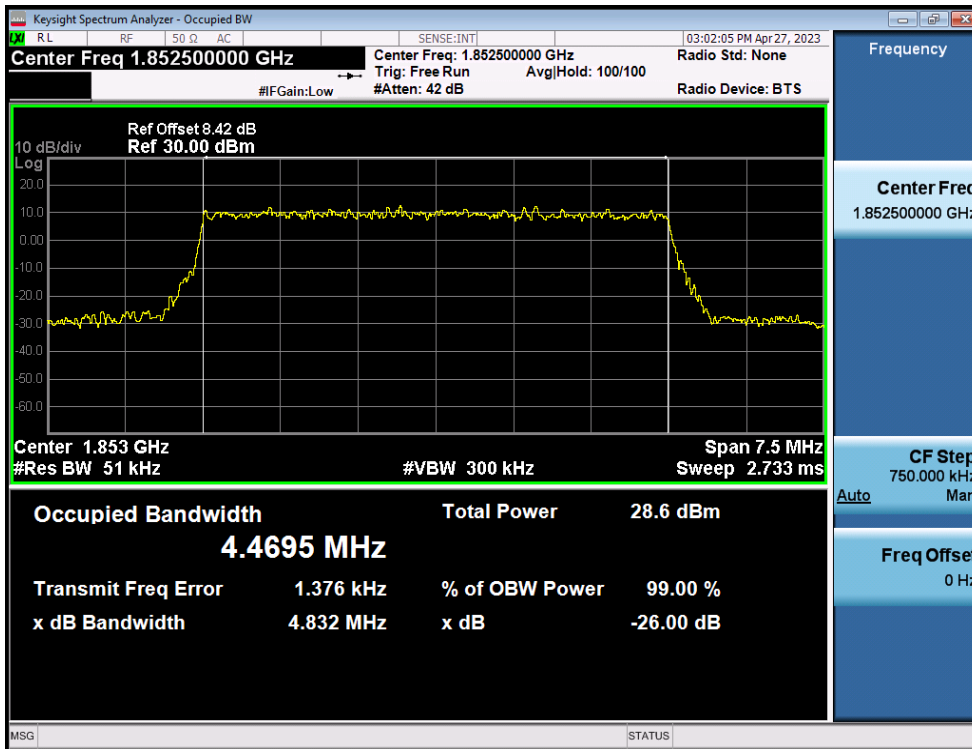
LTE Band 25(2) / 5MHz / 16QAM - RB Size 25
