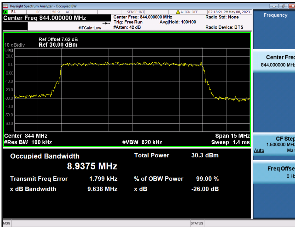
LTE Band 26(5) / 10MHz / QPSK - RB Size 50
