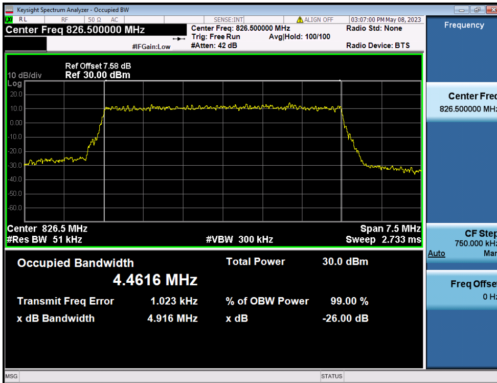
LTE Band 26(5) / 5MHz / QPSK - RB Size 25
