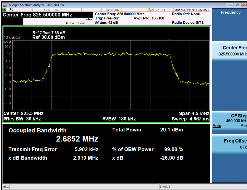
LTE Band 26(5) / 3MHz / 16QAM - RB Size 15
