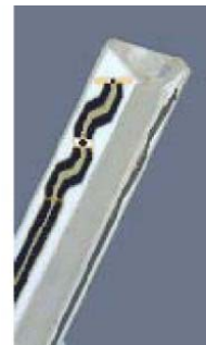
Figure E.2.2 Probe Thick-Film Technique
