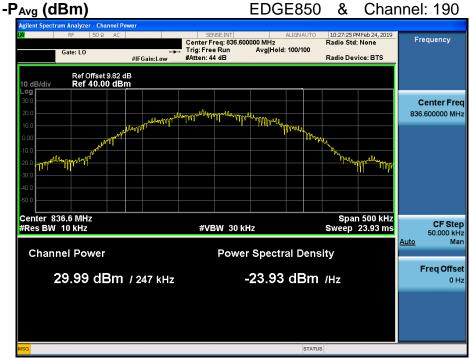
$PAPR (dB) = P_{Pk} (dBm) - P_{Avg} (dBm) = 33.28 dBm - 29.99 dBm = 3.29 dB$
