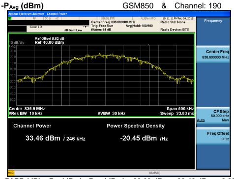
PAPR (dB) =  $P_{Pk}$  (dBm) -  $P_{Avg}$  (dBm) = 33.69 dBm - 33.46 dBm = 0.23 dB
