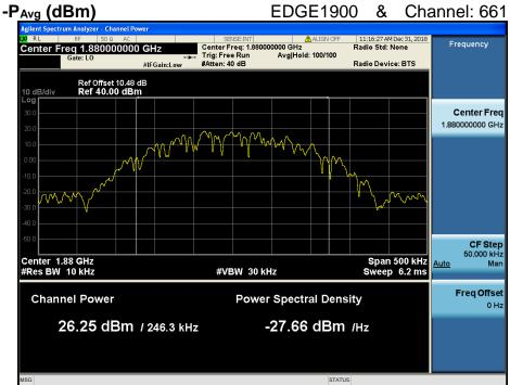
$PAPR (dB) = P_{Pk} (dBm) - P_{Avg} (dBm) = 29.95 dBm - 26.25 dBm = 3.70 dB$
