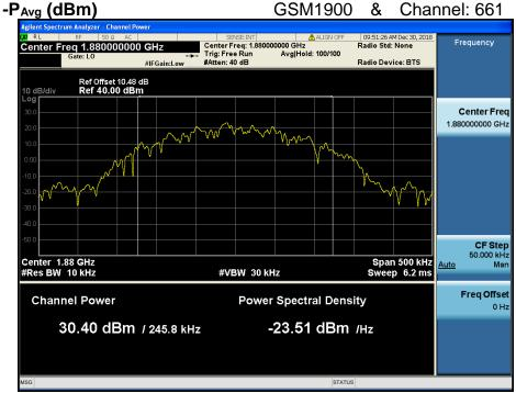
$PAPR (dB) = P_{Pk} (dBm) - P_{Avg} (dBm) = 30.50 dBm - 30.40 dBm = 0.10 dB$
